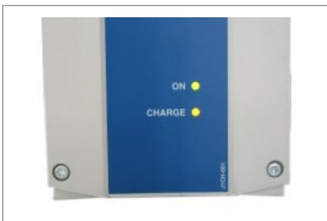
Fig. 2 Indicator light ON and CHARGING
