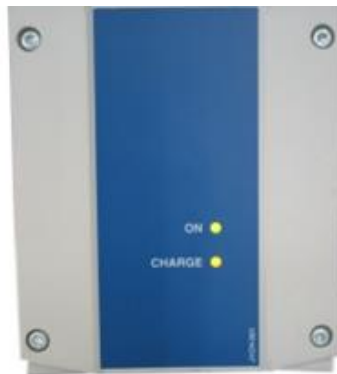
ON = power ON CHARGE = battery CHARGING
